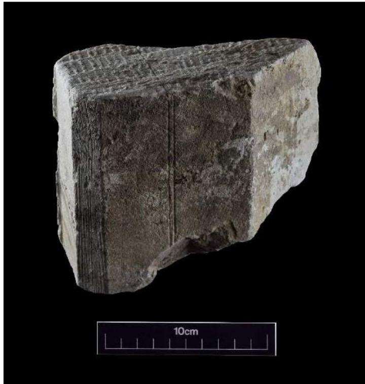
Plate 6: Voussoir stone (SF.6) displaying evidence of claw tooling, scale 0.1m. Photography by C. Casswell
